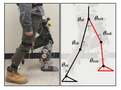
Fig.8 7-links Robotic Model
