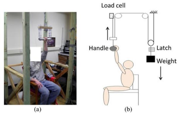
Fig. 2. Experimental setup. (a) Subjects were instructed to sit in a chair with the hand resting on the handle. (b) At a random time, the latch was released, dropping the weight (20% of each subject's hand strength), which applied sudden upward force to the handle. The subjects were instructed to stabilize the handle as soon as they noticed the perturbation.
