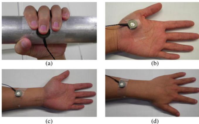
Fig. 4. Four skin sites for noise were (a) middle fingertip, (b) thenar eminence, (c) volar forearm, and (d) dorsal forearm. For the fingertip location, the vibrotactile device was embedded into the handle (a).
