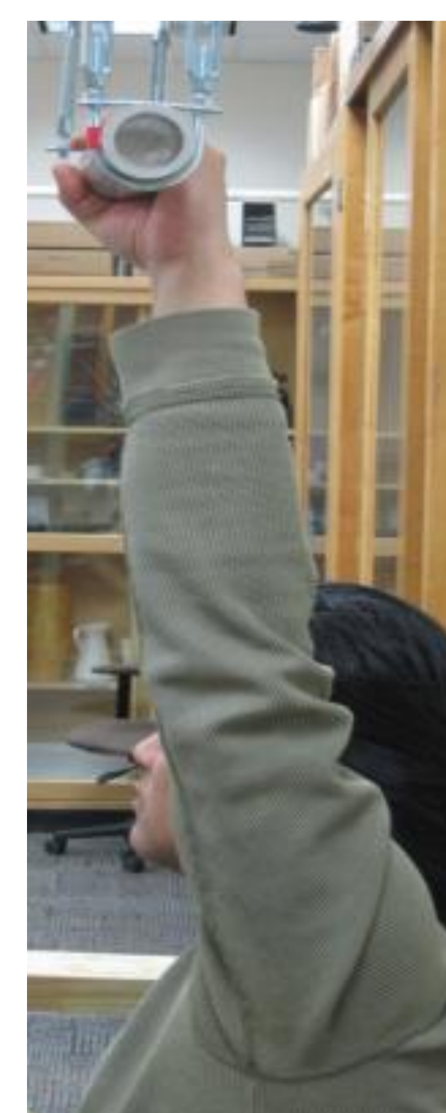
Fig 2. Experimental setup. The handle moved up at a random time. The subjects were instructed to stop the handle as soon as they noticed perturbation.
