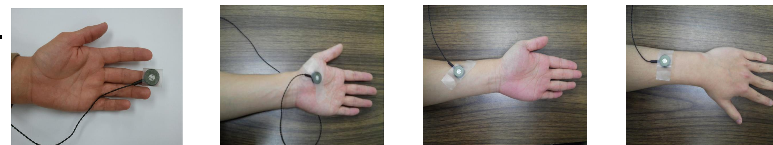
Fig 3 Vibrotactile device (C-3 Tactor, Engineering Acoustics, Inc., Casselberry, FL).
