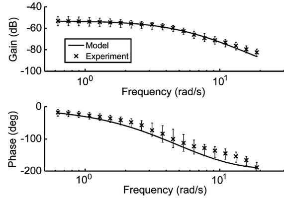
Fig. 4. Example of Bode plots of the frequency response function (FRF) from experimental data of a young adult ( $\times$ ), sensitivity function (solid line) which best fit the FRF. Error bars represent one standard deviation. Experimental data are averaged over ten FRF of a single subject.
