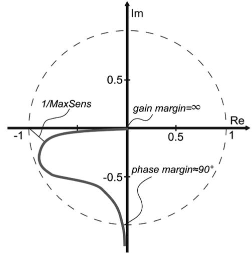
Fig. 1. Sample Nyquist plot illustrating a situation when gain margin and phase margin measures incorrectly suggest a very robust and stable system. Gain margin is infinity and phase margin is  $90^\circ$ , yet this system is very close to instability because the open-loop transfer function (grey) nearly encircles the critical point  $-1$  as indicated by the small  $1/MaxSens$ . (Encirclement of the critical point indicates an unstable system.)
