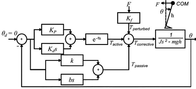
Fig. 2. Block diagram of the postural control system in the Laplace domain. PD control with time delay, passive torque generator, and unity sensory feedback were used. Total corrective torque,  $T_{\text{corrective}}$ , is sum of torque from active control,  $T_{\text{active}}$ , torque from passive control,  $T_{\text{passive}}$ , and torque from the impulsive perturbation,  $T_{\text{perturbed}}$ .
