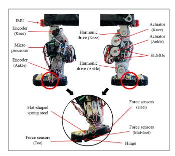
Fig. 3. AMPRO II-a custom-built powered transfemoral prosthesis
