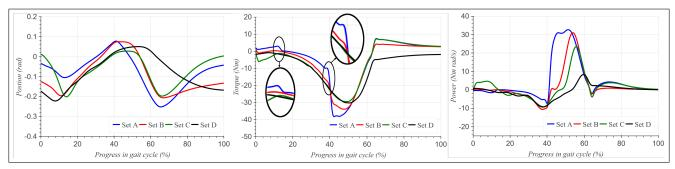
Fig. 4. Averaged results of the experiments. Left: Ankle angle, Middle: Ankle torque, and Right: Ankle power. The sections of the torque curve corresponding to foot-drop and heel-off have been enlarged.
