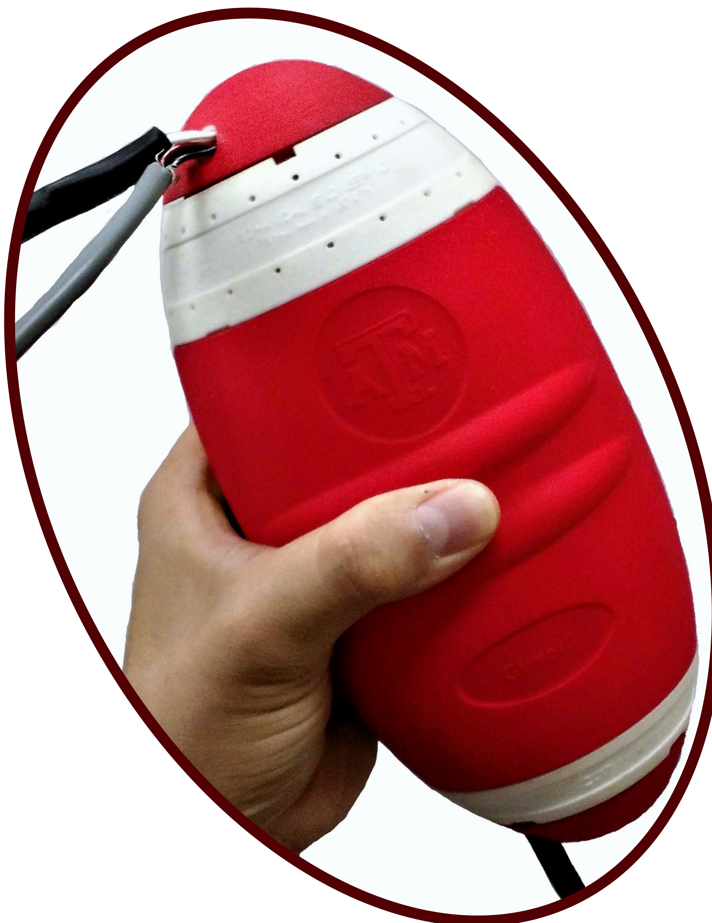
Fig. 1 Image of the Gymball being gripped by a human hand. Finger holds facilitate the user to grip the device comfortably.
