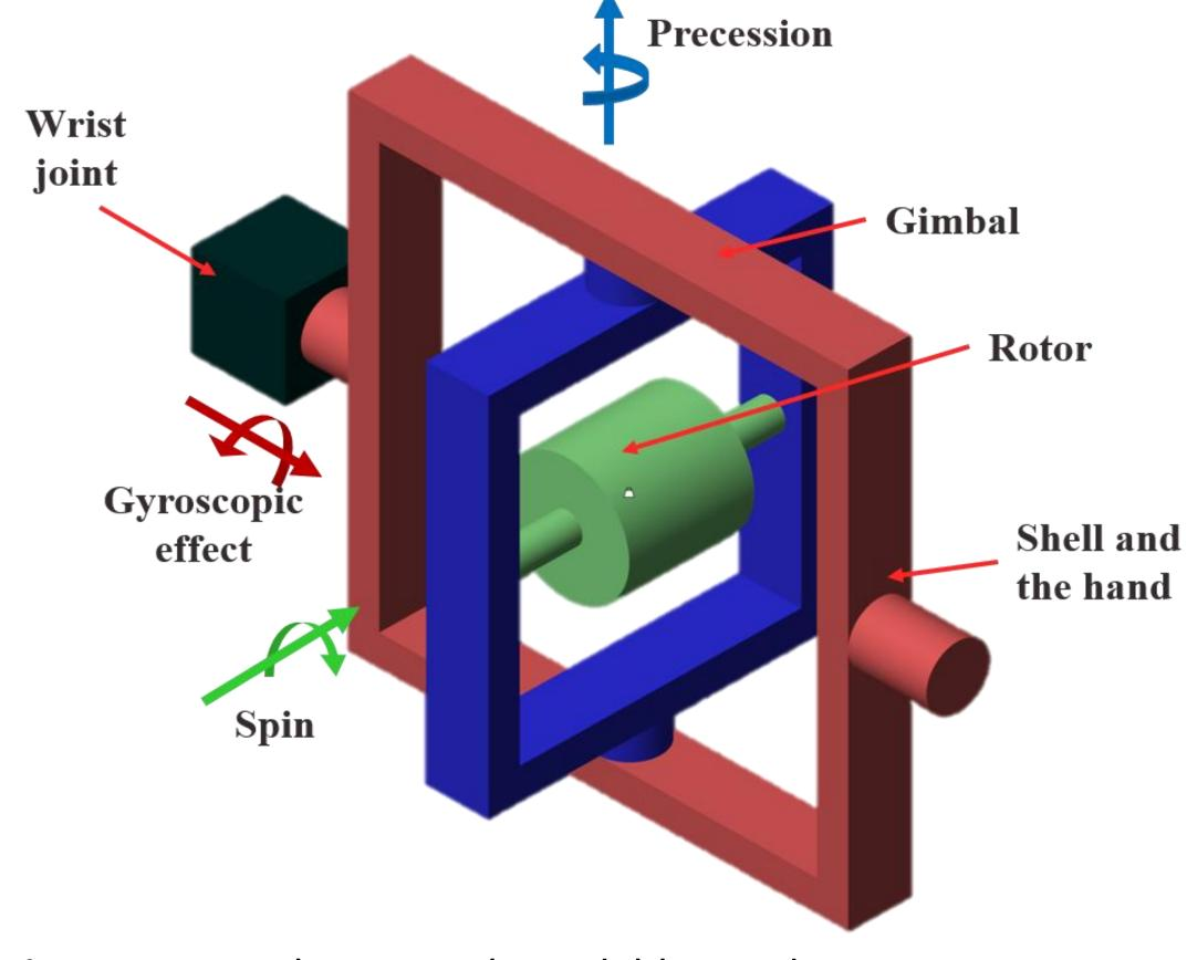
**Fig. 1** Device schematic: the red, blue and green components represent the user's hand, gimbal and the rotor, respectively.
